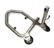
1. Pull right pin out and rotate right arm up
