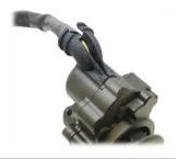
**9** - Fit the clamp loosely with the 2 x M5 screws and slide the new assembly over the end of the handlebar and into position.
