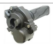
**8** – Stretch the rubber O Ring over the main connector and slide it up near the twist grip housing. Now fit the wire exit guard as seen in these images and hold them together using the O ring.
